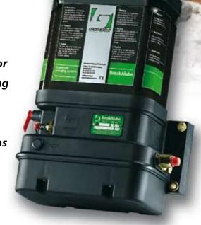
BreakAlube is based on Groeneveld's proven TriPlus progressive grease pump. Vital pump parts, including pump element and drive axle bearings, are entirely new developments. BreakAlube can build up working pressures up to no less than 275 bar and can be used with greases up to NLGI Class 2 including additives such as graphite and copper.
