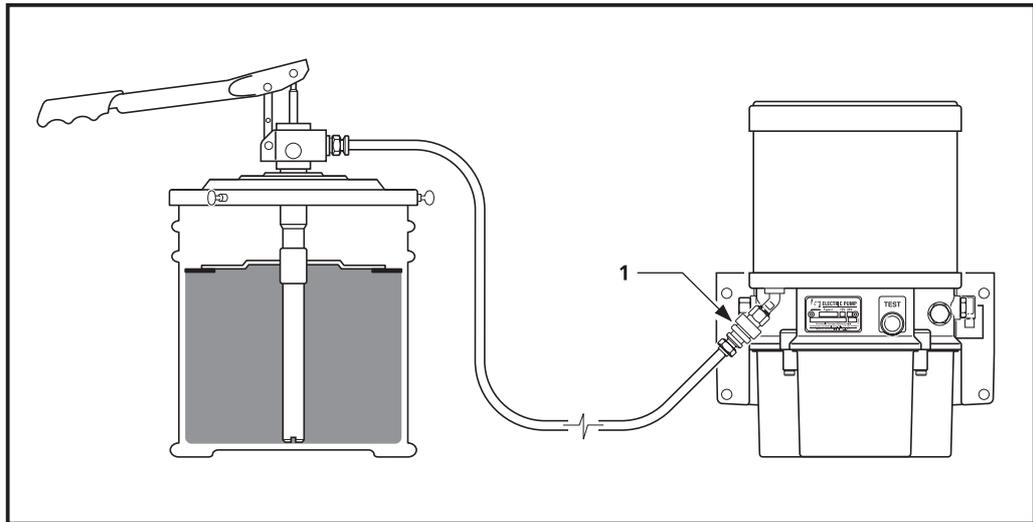
Figure 10.1 Filling the grease reservoir
