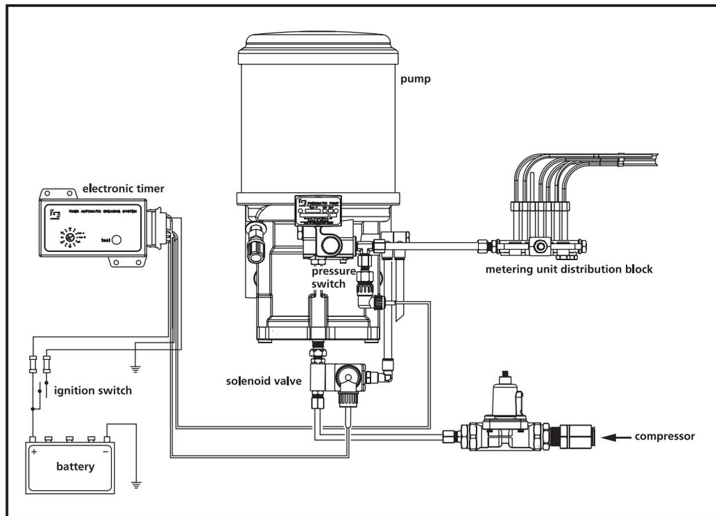
Figure 4.1 System with pneumatically operated pump and electronic timer (schematically)
