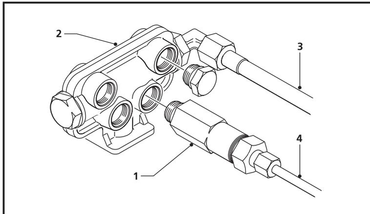
Figure 8.1 Distribution block with metering units
