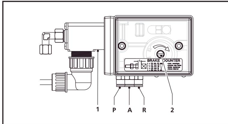
Figure 7.1 Electrically operated brake impulse counter
