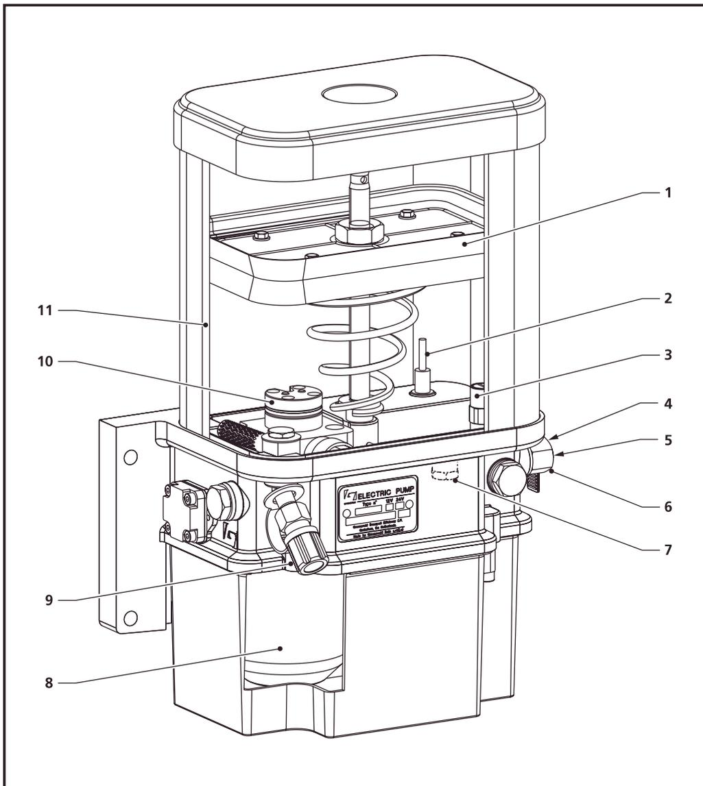
Figure 5.2 Electrically operated pump
