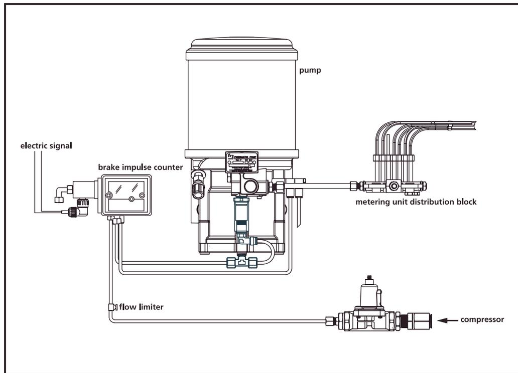
Figure 4.3 System with electrically operated impulse counter (schematically)
