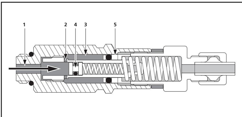
Figure 8.4 Metering unit in phase A
