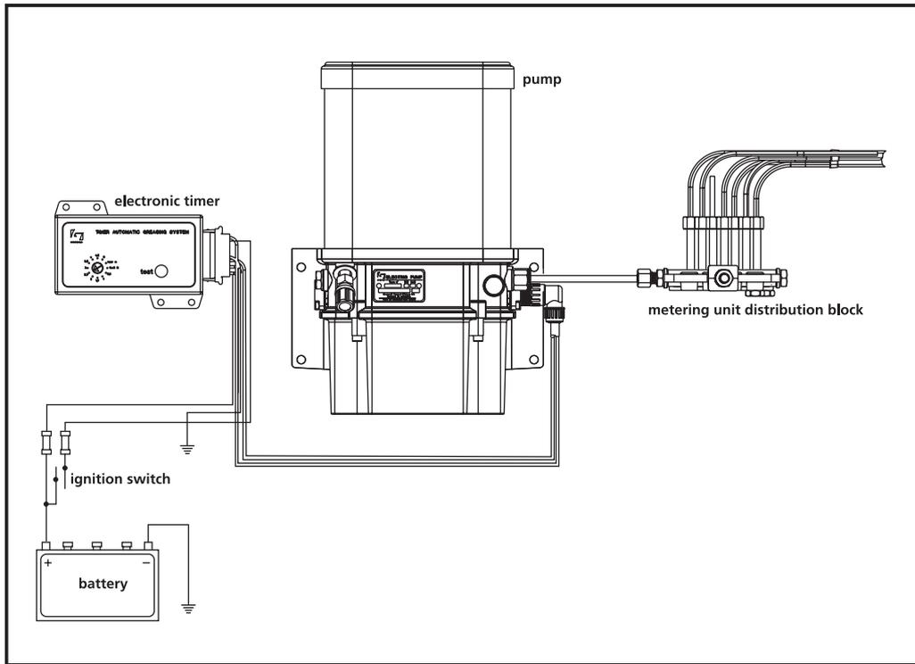
Figure 4.4 System with electrically operated pump (schematically)
