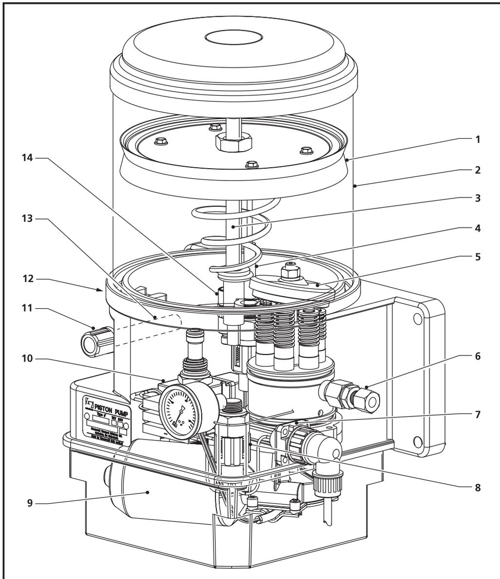
Figure 5.3 The electric plunger pump
