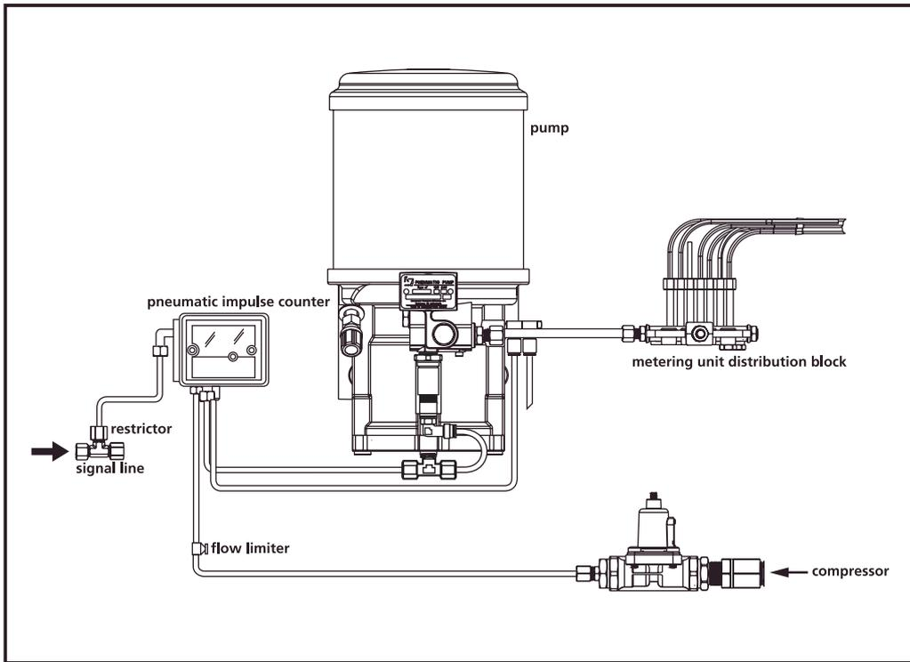
Figure 4.2 System with pneumatically operated impulse counter (schematically)
