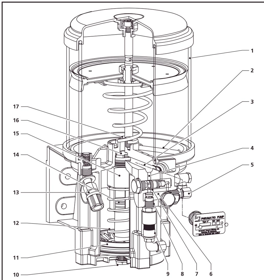
Figure 5.1 Pneumatically operated pump
