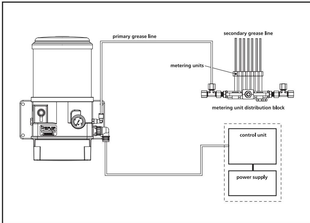
Figure 4.5 System with electric plunger pump (schematically)
