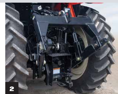
[1] PTO [2] 3-point hitch, category III, shown with opt. Quick Hitch.
