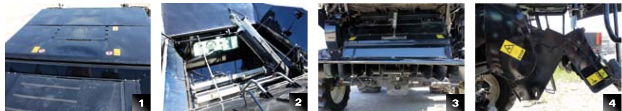
[1] Grain tank in closed position [2] Open / extended grain tank [3] Chopping position [4] Swath position
