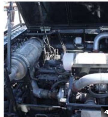
[1] Rear access area [2] Large easy to use latches [3] Cooling system service access [4] Engine compartment.
