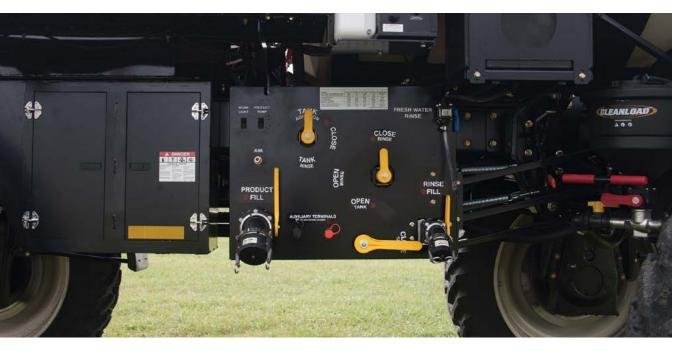
**FILL STATION** The operator/product load station is well-labeled with large clear instructional decals and logical valve orientations. All points easily accessible from the ground for safety and to reduce refill time.
