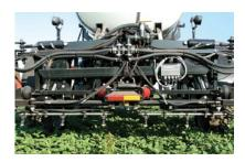
With the ProAction-Flex Boom, you're able to tilt and/or lock the full length of the boom in place, keeping it parallel with the terrain while maintaining proper distance from the spray tip to target. In fact, it's so strong and finely balanced; you can turn at speed without it dipping into the crop.
